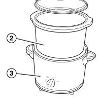
The Control Knob on the slow cooker offers Low and High temperature settings for cooking. The **Keep Warm** setting is for holding the prepared recipe at a perfect serving temperature.
